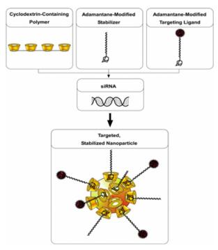
The surface-modifying agents have terminal adamantane groups that form inclusion complexes with the cyclodextrin and contain poly ethylene glycol (PEG) to endow the particles with properties that prevent aggregation, enhance stability and enable systemic administration. Targeting molecules can be covalently attached to the adamantane-PEG modifier, enabling the siRNA-containing particles to be targeted to tissues of interest.
